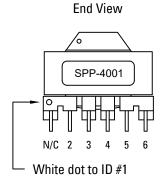
Prem's SPP-4001 is a switchmode, through-hole PCB-mounting transformer. It is designed to be used with a Power Integrations TOP258PN (*TOPSwitchHX* family) integrated chip in a 35 W AC-to-DC flyback for an LCD monitor power supply application.
